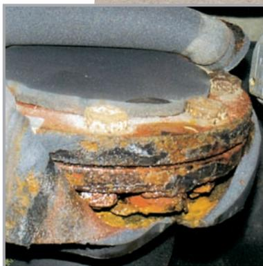
In addition the underlying structures are frequently subject to wear due to the leaking rusty water from these flange connections.
